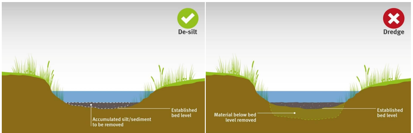
Figure 2: Difference between a de-silt and a dredge
